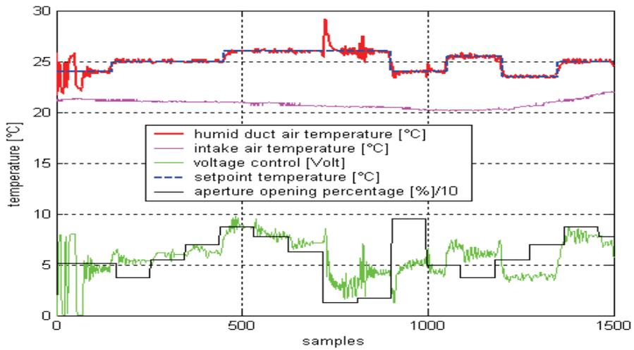
Fig. 6. IAGPC of the air humid duct temperature
