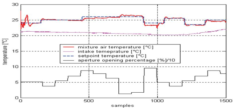
Fig. 8. IAGPC of the air mixture duct temperature
