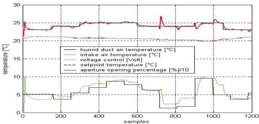
Fig. 10. DAGPC of the air humid duct temperature
