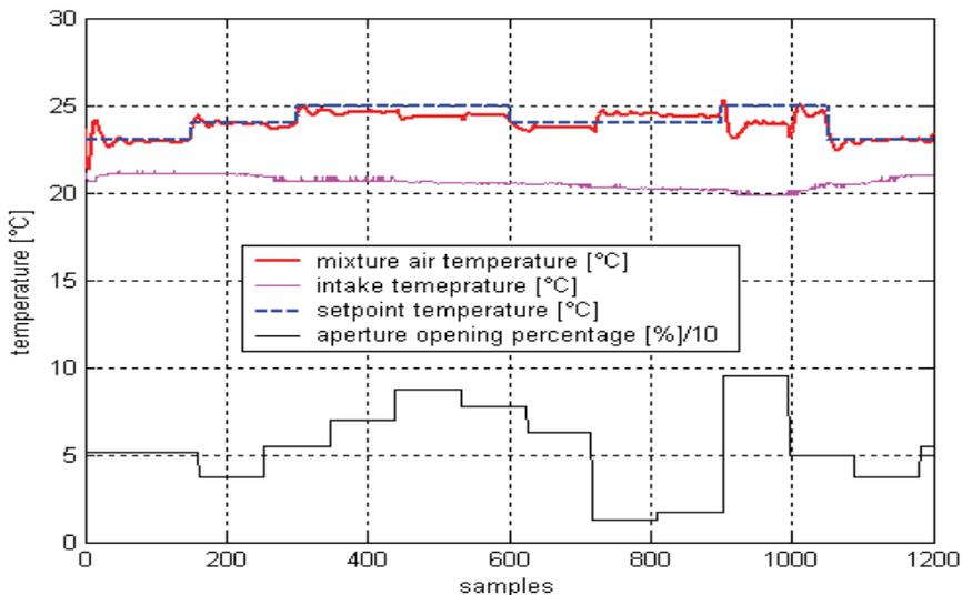
Fig. 11. DAGPC of the air mixture duct temperature
