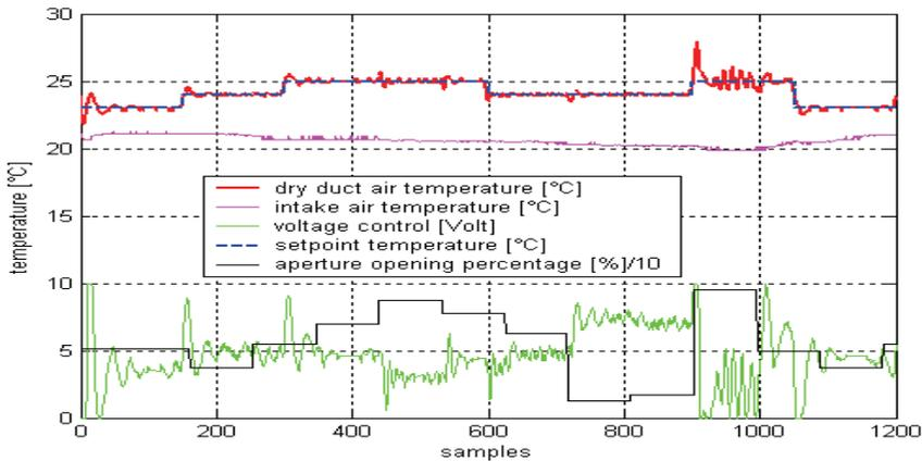
Fig. 9. DAGPC of the air dry duct temperature
