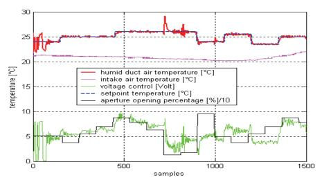
Fig. 6. IAGPC of the air humid duct temperature
