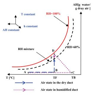
Fig. 1. Thermodynamic cycle of the unit
