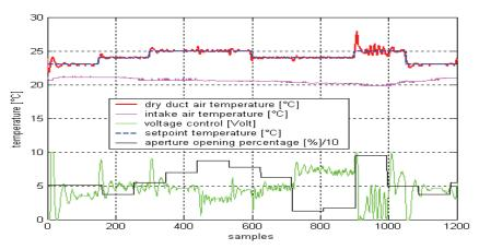
Fig. 9. DAGPC of the air dry duct temperature
