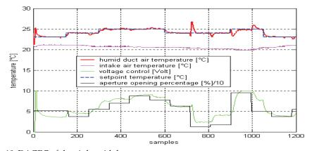
Fig. 10. DAGPC of the air humid duct temperature
