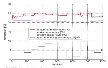
Fig. 11. DAGPC of the air mixture duct temperature
