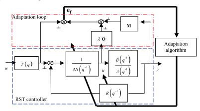
Fig. 3. Equivalent structure of the DAGPC
