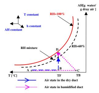
Fig. 1: Thermodynamic cycle of the unit
