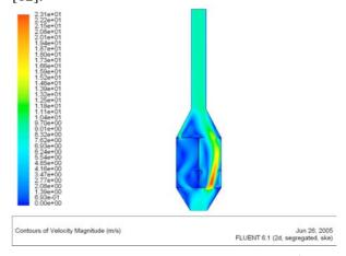
Fig. 2. Contours of velocity magnitude m s<sup>-1</sup> (inlet velocity 8 m s<sup>-1</sup>, opening 10%-90%)
