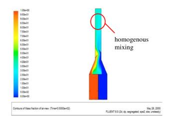
Fig. 4. Device with baffles: Contours of mass fraction of air, inlet velocity 4 m s<sup>-1</sup>, opening 20%-80%.
