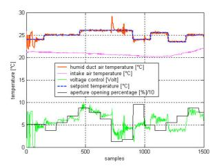
Fig.8. IAGPC of the air humid duct temperature
