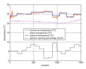
Fig. 10. IAGPC of the air mixture duct temperature
