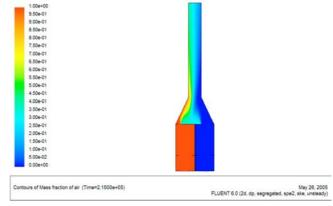
Fig. 3. Contours of mass fraction of air, inlet velocity 4 m s<sup>-1</sup>, opening 20%-80%.
