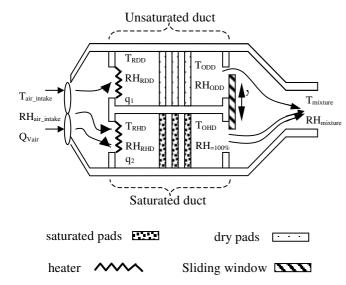
Fig. 5 Cross section view of the air-conditioning unit
