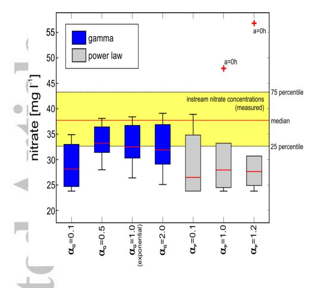
Figure 9: Observed in-stream nitrate concentrations and the nitrate concentration in the missing water source (e.g. farm drains) estimated for the different RT distribution scenarios.
