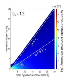
Figure 5: Simulated hyporheic nitrate removal efficiencies for the generic river reach using different parameter sets for mean resident times  $\tau_m$ , threshold factors *a* and shape factors  $\alpha_P$  for power law RT distribution models. The blanked areas above the 1:1 line result from an  $A_r$  factor lying close to zero resulting in a singularity when Equation 2 is calculated.
