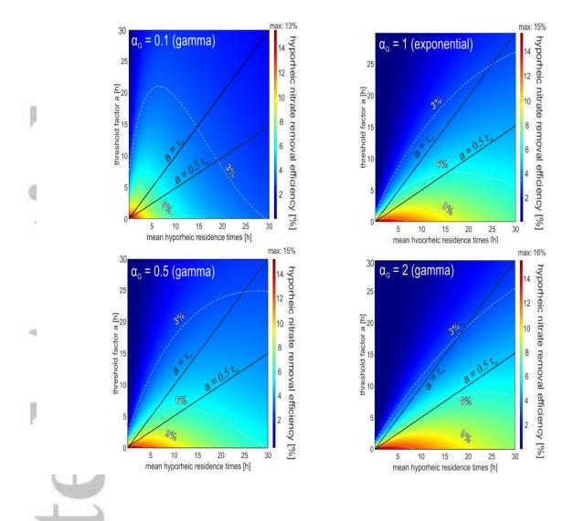
Figure 4: Simulated hyporheic nitrate removal efficiencies for the generic river reach using different parameter sets for mean resident times  $\tau_m$ , threshold factors *a* and shape factors  $\alpha_G$  for gamma-type RT distribution models. Note where the gamma parameter  $\alpha_G$  is 1 it is equal to an exponential distribution.
