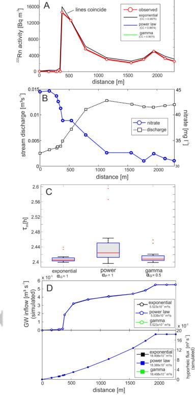
Figure 6: Simulated and observed in-stream <sup>222</sup>Rn activity (A); measured discharge and in-stream nitrate concentrations (B); Box-Whisker-Plots for the simulated mean hyporheic RT shown for the exponential ( $\alpha_G = 1$ ), gamma-type ( $\alpha_G = 0.5$ ) and power law ( $\alpha_P = 1$ ) distribution (C); modeled cumulative groundwater inflow and cumulated steady-state hyporheic water flux (D).
